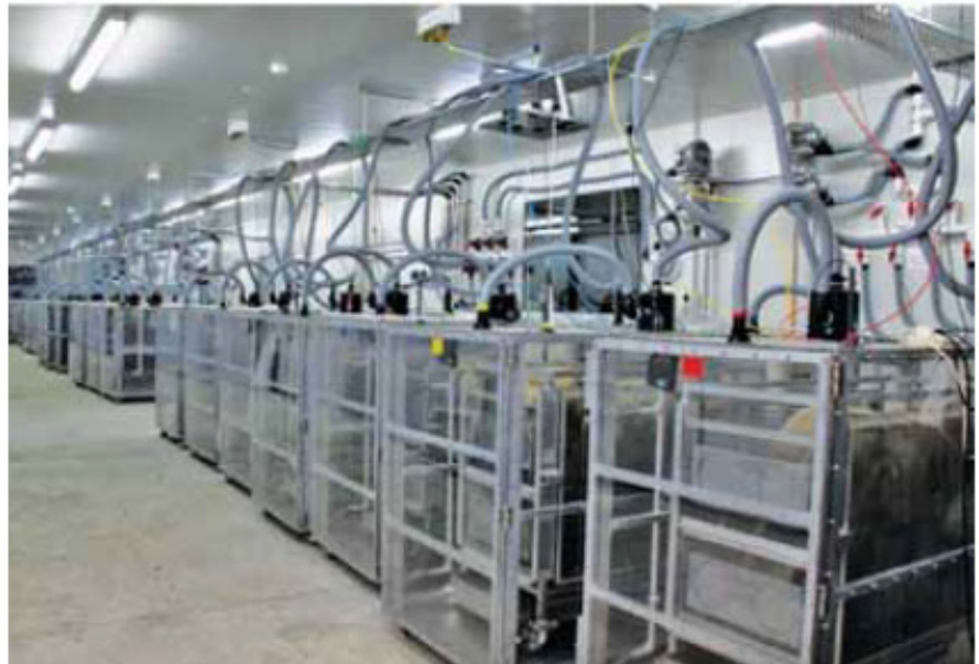
Plate 1: The sheep respiration facility comprises 24 chambers housed in a dedicated building.
