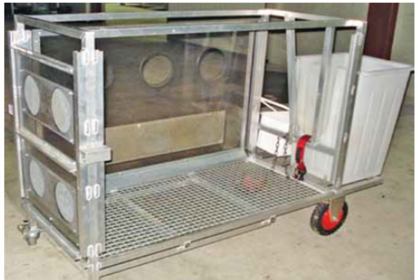
Plate 4: A modified metabolic crate used to hold the sheep in the respiration chamber.
